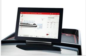
The software shows the difference between the depths read and the depths defined by the manufacturer
