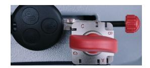
Sides C and D: for keys to be cut on both sides and locked on the groove
