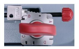
Side B: for keys placed on their rear needing cuts with a depth of less than 3.9mm
